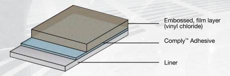
The picture above shows a typical DI-NOC™ Architectural Finish composition. Composition and materials vary for different product lines.
